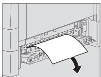
⚠ If it is difficult to find or remove the misfed paper, open the drawer of the Paper Feed Unit.
