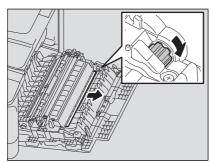
If you cannot see the misfed paper or it is difficult to remove, open the drawer in which you have loaded paper and remove it.
