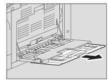
• Depending on its condition, paper may not be fed for bypass copying. In this case, turn over the paper and place it again as shown in the figure.
