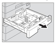
Pull out the trailing guide while pushing its lower part to the direction of the arrow. Then reinstall the guide at the position of the desired paper size.
