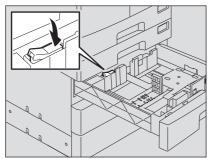
While pushing the green knob of the side guides, adjust the side guides at the position of the desired paper size.
