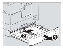
5 Check that the guide width is correct, there is no folded/curled paper or overloading, and then close the drawer.
