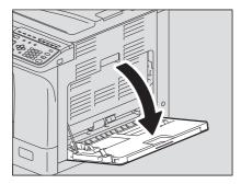
Pull the paper holding lever out, and then load paper face down and straight on the bypass tray.
