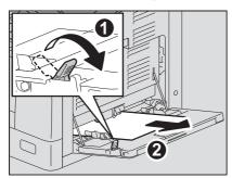
Check beneath the transport guide inside of the side cover. Check if any paper is misfed under the transport guide behind the transfer unit. P.195 "Paper misfeeds inside of the side cover"
