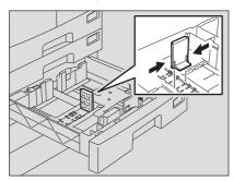
The paper size is indicated on the bottom inner surface of the drawer.
